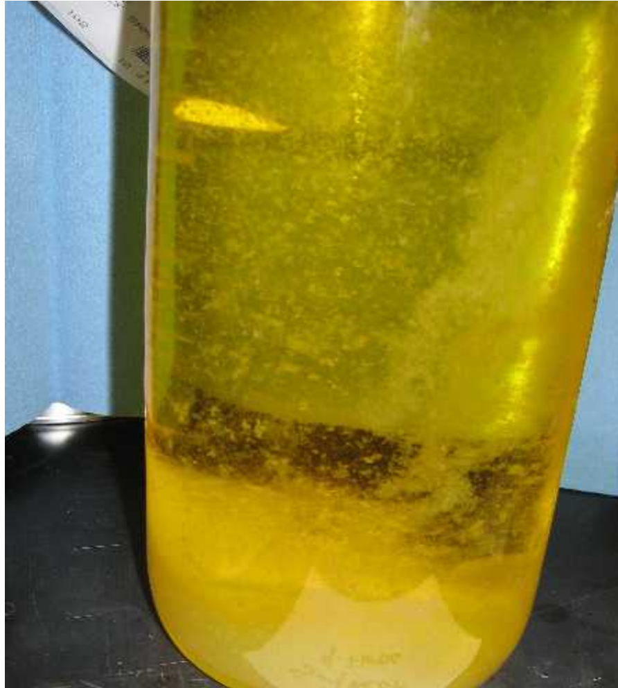
B100 with 32 F Cloud Point Held for Several Days at 48 F
