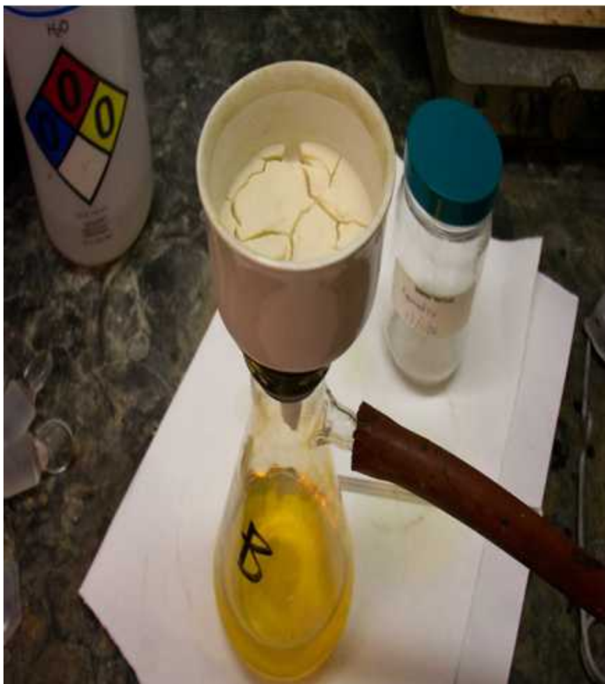
Filter Cake from Filtration of Acetone Extract (After Acetone Evaporation).
