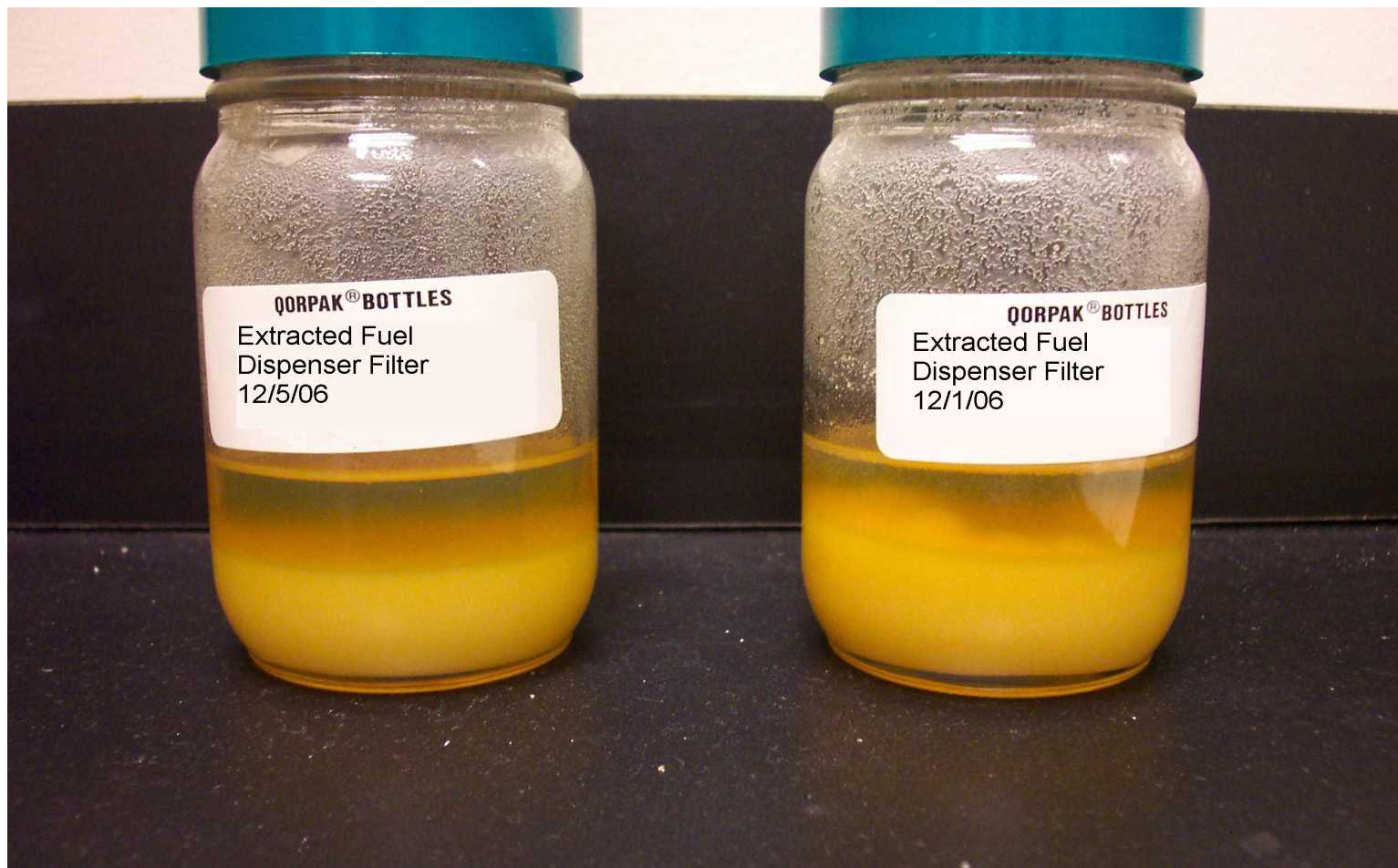
Acetone Free Extract of Plugged Dispenser Filters At 40 F
