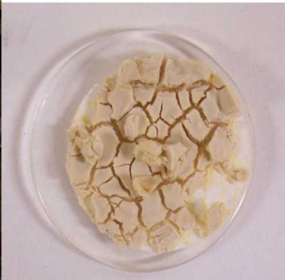
Filter Cake from Filtration of Acetone Extract (After Acetone Evaporation).
